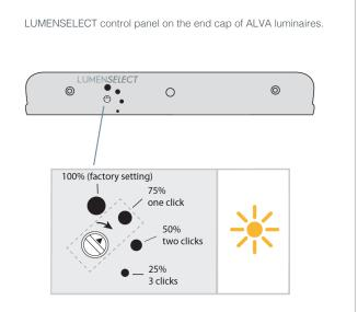
The LumenSelect rotary switch should be turned gently clockwise with a small flathead screwdriver with a 1/8" or 3mm wide tip, one click at a time from factory setting to get desired output level.
